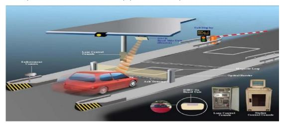
Figure 5: ETC System working principle
