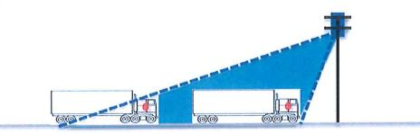
Here the 5 GHz RLAN transmitters are found inside the vehicle. If the RLAN device is transmitting within the TTT communication zone, its transmission would radiate through the vehicle window interfering directly with uplink communications to the TTT road side receiver antenna. In the case of a cabriolet or a motor cycle there is no wind screen, which normally reduce transmit power by 3 dB.
