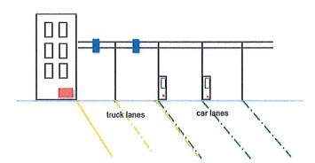
The 5 GHz RLAN transmitter is situated close to the TTT system. The figure above shows an example with a multilane road toll. The 5 GHz RLAN transmitter appears in red and the TTT receivers are shown in blue. In this scenario it is assumed the 5GHz RLAN transmitter, access point or the device, is close to the TTT communication zone, but situated inside a building. The distance between the 5 GHz RLAN transmitter and the TTT road side receiver antenna is assumed to be 4 m or longer.
