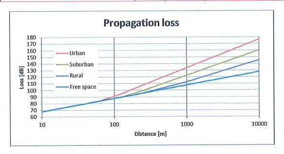
The figure above describes attenuation of the different propagation models.
