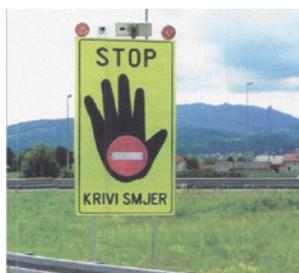
Article 22 of the Book of regulations says that the road danger sign should be expanded with an additional board explaining the type of threat. When used on the LED traffic/VMS sign, the additional information provided is textual, limited to 7 letters or symbols entry. If there is no adequate description of the specific road danger, the Book of regulations assigns the word «OPREZ» (Eng. «CAUTION») which still does not specify the type of danger.
