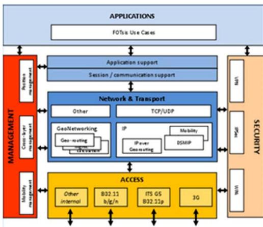
The conceptual framework of the FOTsis architecture is the ETSI ITS Station. It integrates the concepts necessary to help bring to life the general idea of Cooperative Systems into a set of modules covering a whole communications and applications stack and which, as a whole, will provide the capabilities to meet the requirements of Cooperative Systems and Services.
