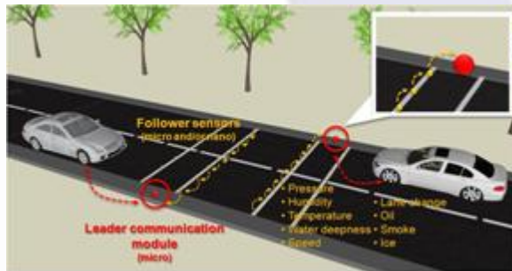
Smart Strip miniaturised multi-sensorial platform at a highway or rural environment.
